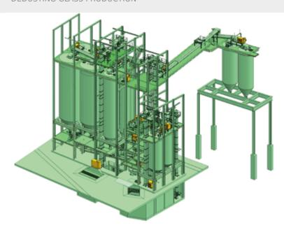
In a batch plant the required raw materials for glass production are stored in silos, from there charged into container scales and weighed according to the later glass composition. Afterwards the raw materials are mixed and transported to the glass melter via conveyor belts or buckets.
