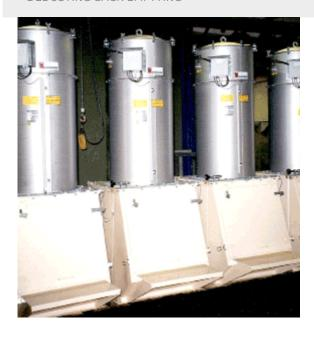
20 sack emptying filter, existing out of sack discharge and a **cartridge filter**cleaned by compressed air, were delivered. All sack emptying stations are centrally exhausted by a single fan. The pneumatic cleaning of filter cartridges is automatically turned on and off by a proximity switch, which is initiated by the filler chute door.
