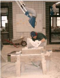
About 20 training workplaces for stonecutters are dedusted by a central filter. The total volume flow amounts to 360 m<sup>3</sup>/min and is cleaned by an **pleated element filter INFA-LAMELLEN-JET, type AJL 3/1083**, with 324 m<sup>2</sup> filter area.
