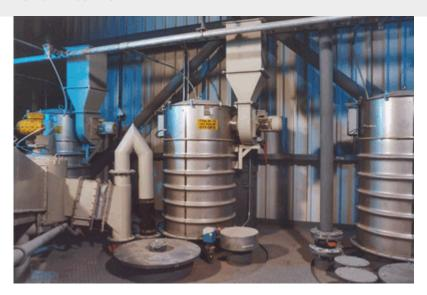
Several silos for cement, pulverised limestone, fly ash and molding sand were installed for a mixing facility in a cement plant.
